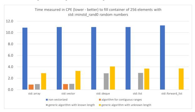
CPE – cycles per element of the container filled with numbers. Measured on Intel® Xeon® Gold 6152 Processor.
