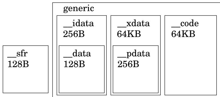
The very common MCS-51 architecture has a large number of address spaces that are accessed in different ways. Objects could be anywhere, so generic pointers contain tag bits to designate the address space they point into. The arrangement is so complex that reads and writes via pointers are implemented as support function calls (unless the optimizer can prove that a particular pointer points into a specific address space at the point of access), and thus expensive.
