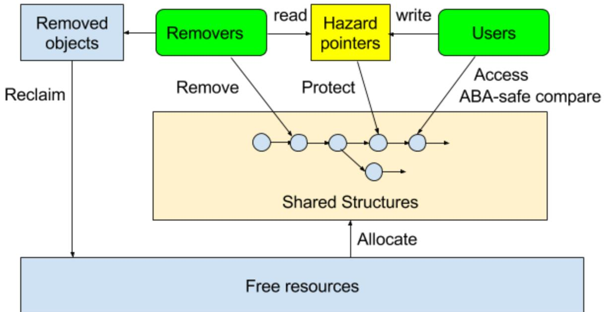
Hazard pointers are owned and written by threads that act as users (i.e., may use removable objects) and are read by thread that act as removers (i.e., may remove objects). The set of user and remover threads may overlap, so the same thread may write to its own hazard pointers when using objects and read the hazard pointers including those of other threads when reclaiming removed objects.
