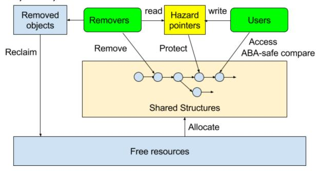
Hazard pointers are owned and written by threads that act as users (i.e., may use removable objects) and are read by thread that act as removers (i.e., may remove objects). The set of user and remover threads may overlap, so the same thread may write to its own hazard pointers when using objects and read the hazard pointers including those of other threads when reclaiming removed objects.
