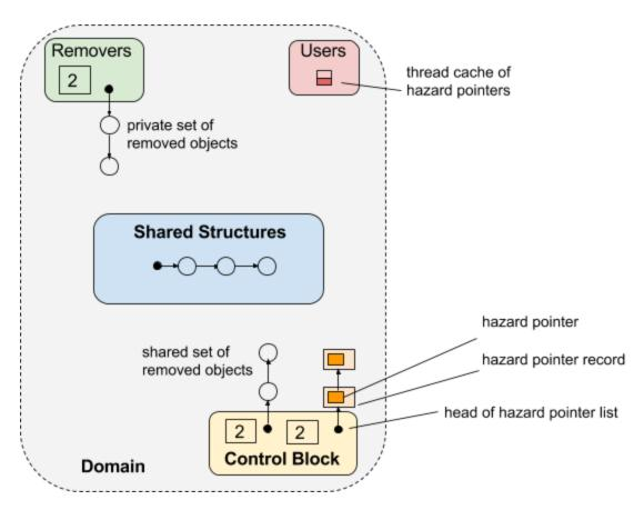
The above diagram shows the main components of the hazard pointer method's design:
