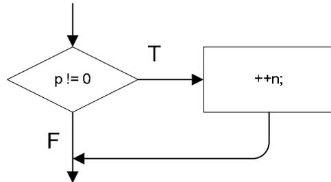
The result of this process is a flow-chart composed of the “little boxes”. Each arrow that flows into a box or out of a box specifies one sequence point. By and large, this much of the sequence-point model is well-understood by programmers and implementers. However, it is only the top-level sequenced operators that produce little boxes in the flow chart; that detail is sometimes not fully understood.
